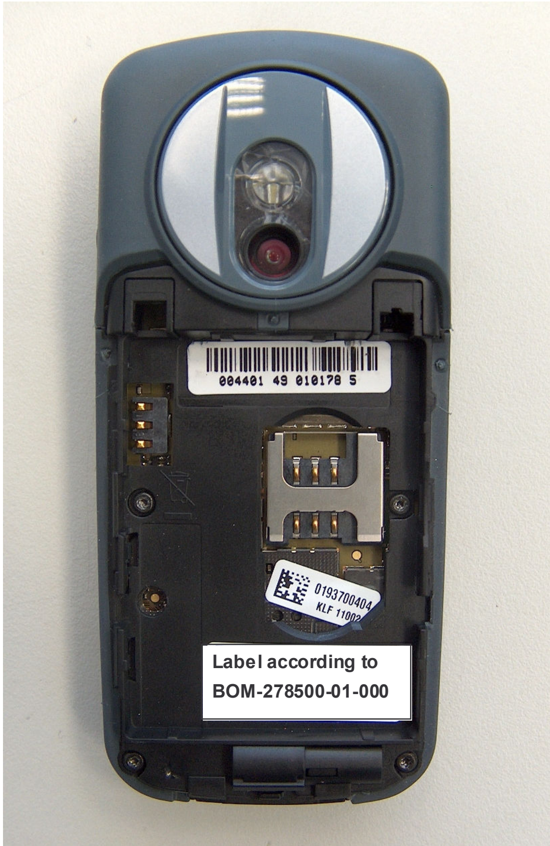
Figure 1 FCC ID and IC ID label position in M81 product from BenQ-Siemens
