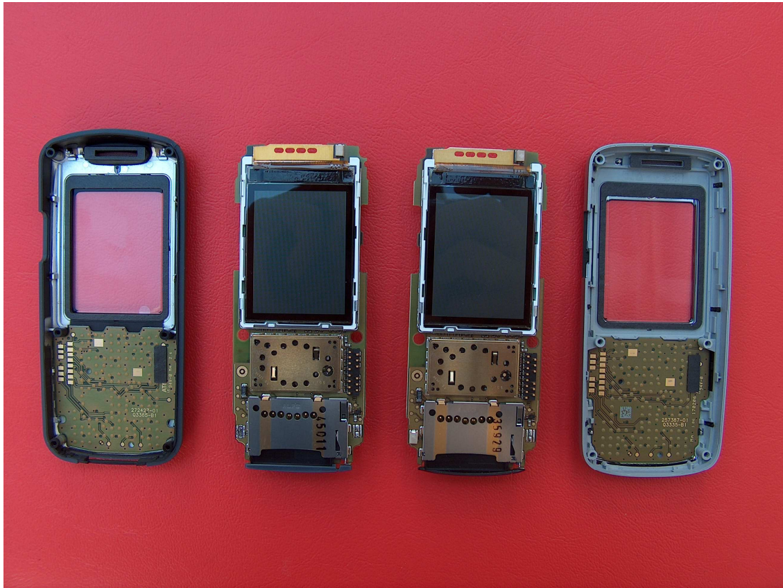
M81 on left side. C81 on right side. Front side of PCB is identical.
