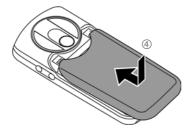
• To remove, press the battery cover ⑤, and slide it off the phone ⑥.
