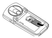
Insert the battery sideways into the phone ②, then press it downwards ③ until it engages.
