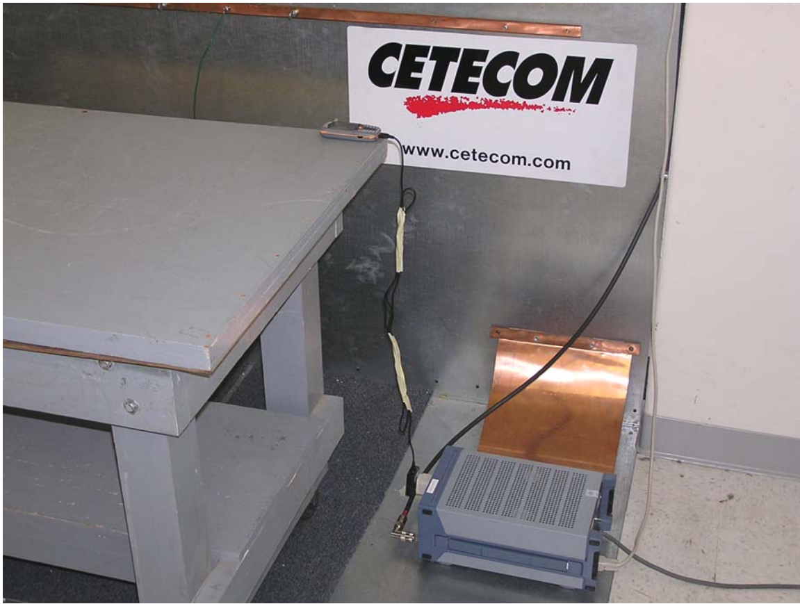
Test setup – AC Line conducted emissions
