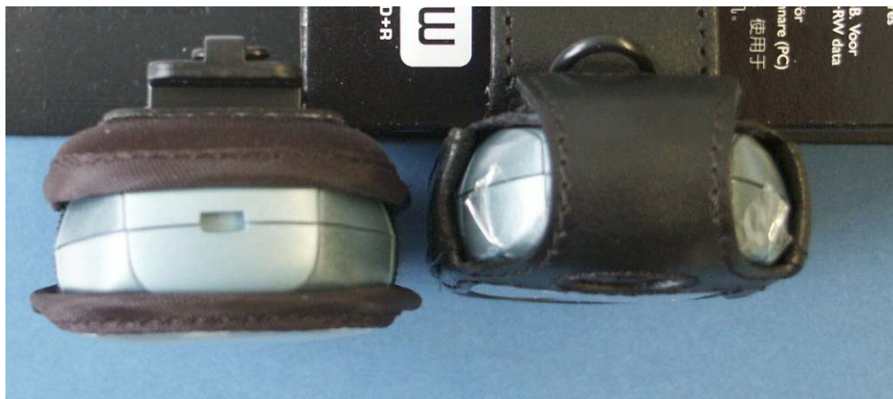
Fig. 22: Picture which show that the leather case FCL-500 (right) provides the smaller distance to the body compared with Loop case FCT 500.
