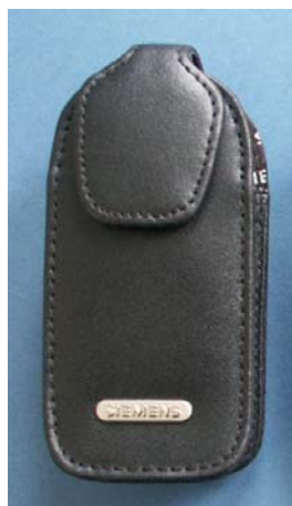
Fig. 23: Additionally available Leather holster FCL-510 which is only a carry case since there are no apertures for a headset or a data cable. Therefore measurements are not required .
