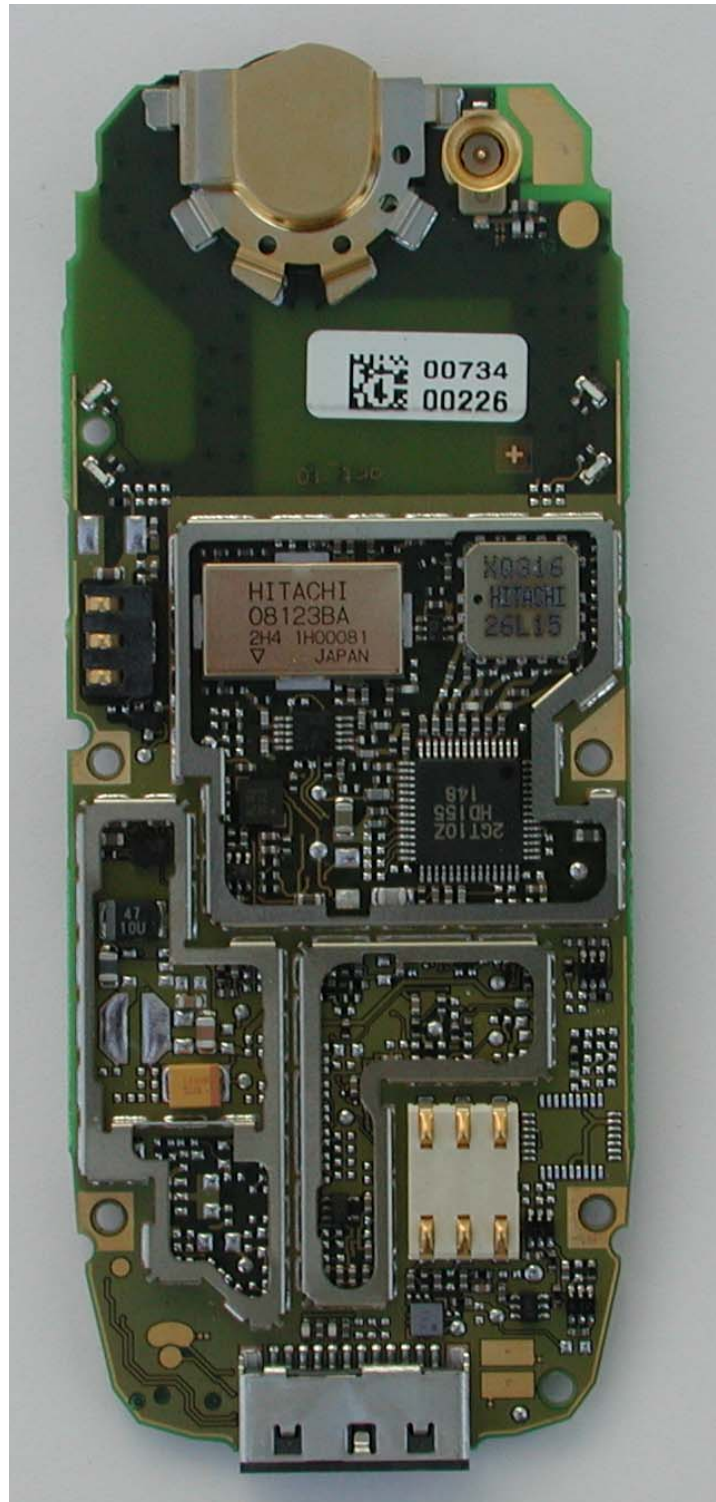
M55 Board without shielding, side 2
