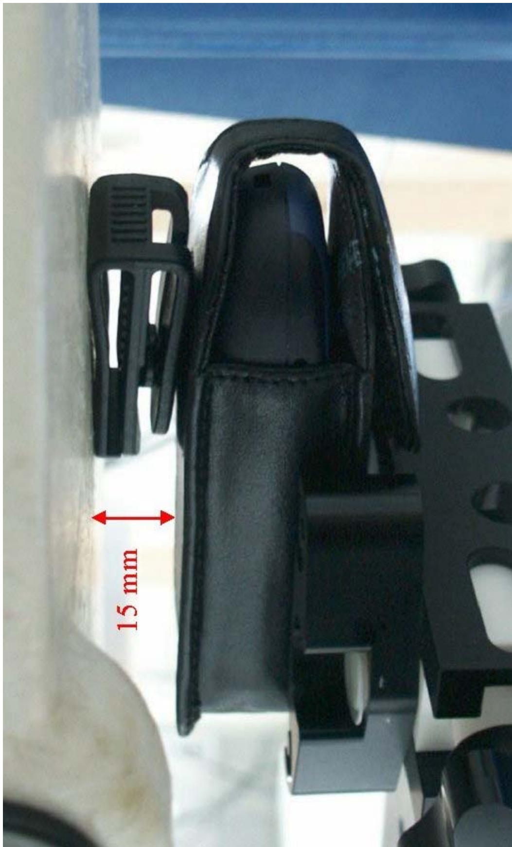
Fig. 5: Body worn configuration with leather case, display towards the ground.
