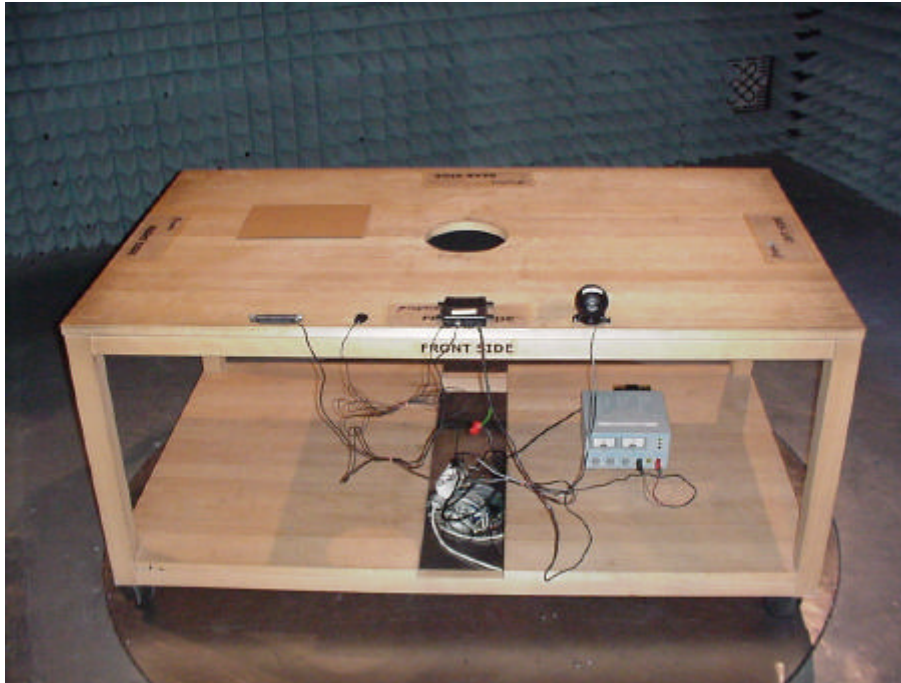
Picture 1 : Setup for radiated emission test
