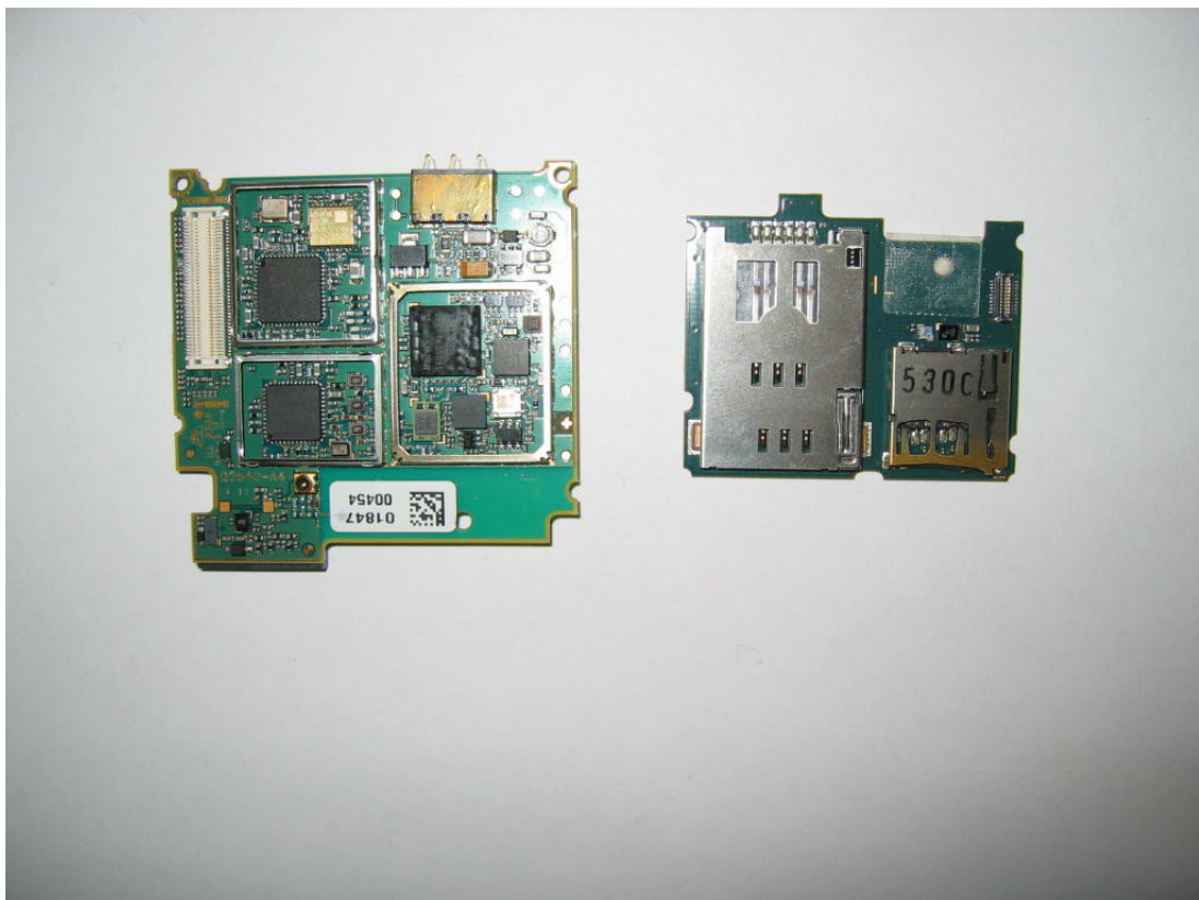
EF81 Main PCB and Card PCB removed shieldings (Back part)
