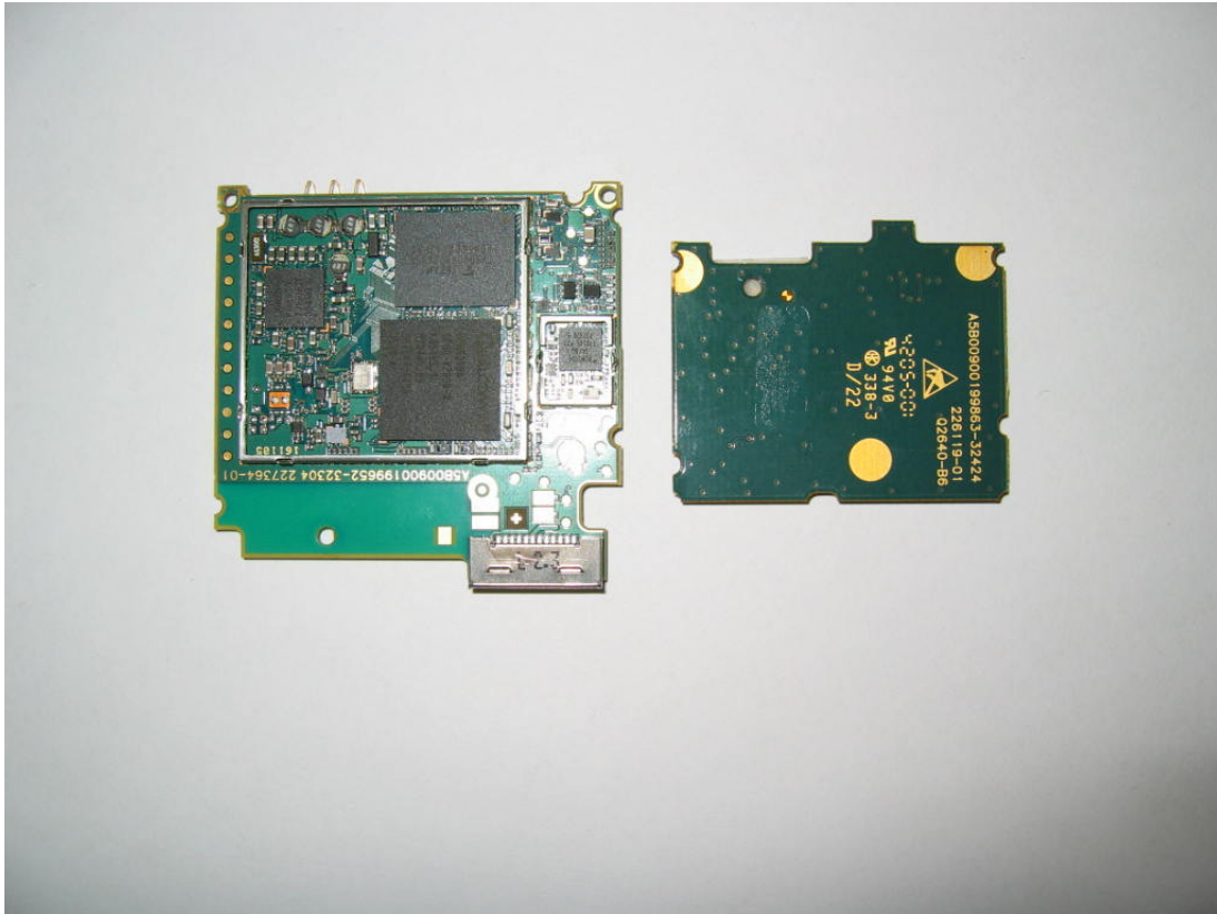
EF81 Main PCB and Card PCB removed shieldings (Front part)
