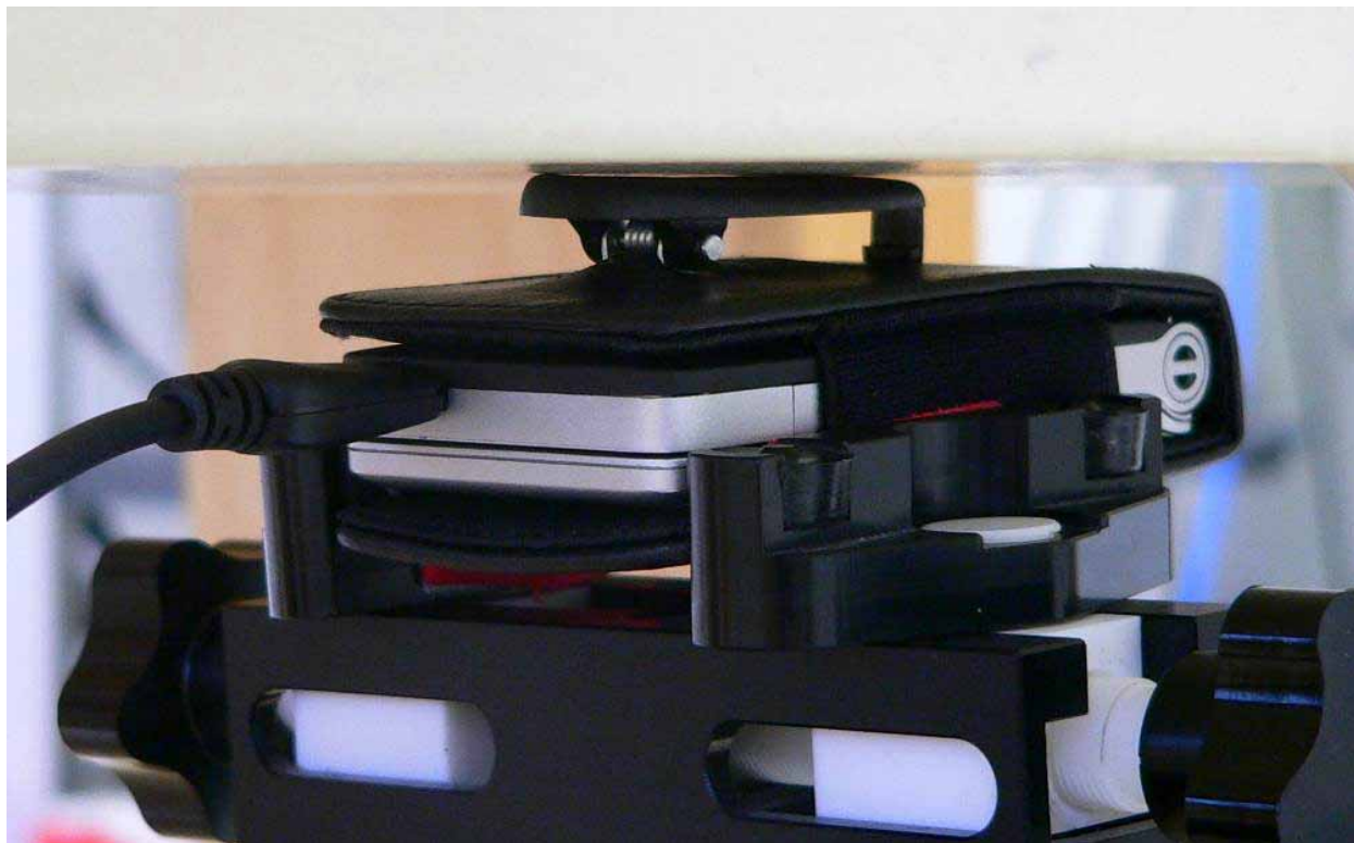
Fig. 26: Body worn configuration, GPRS (Class 10) with data cable and FCL 170 carry case, antenna towards the phantom.
