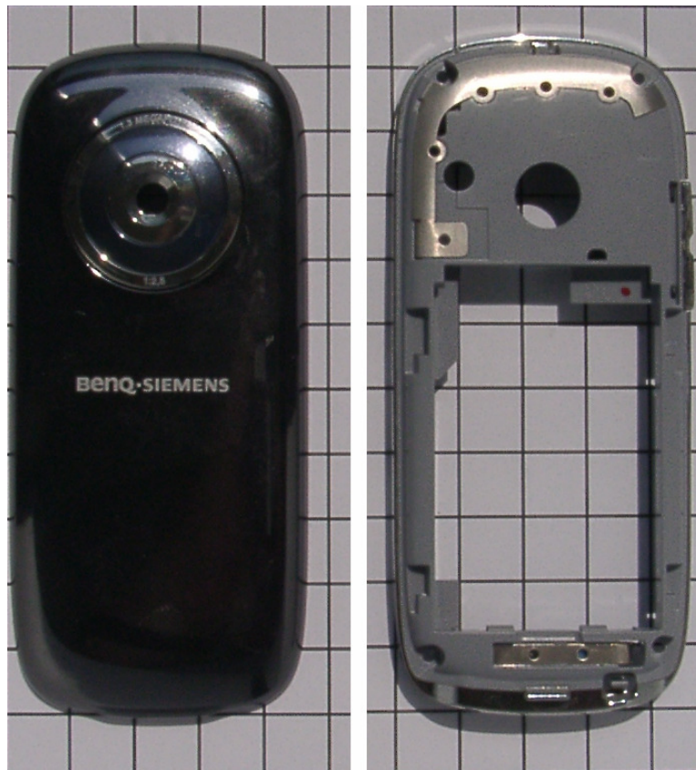
Back cover and back frame with antennas
