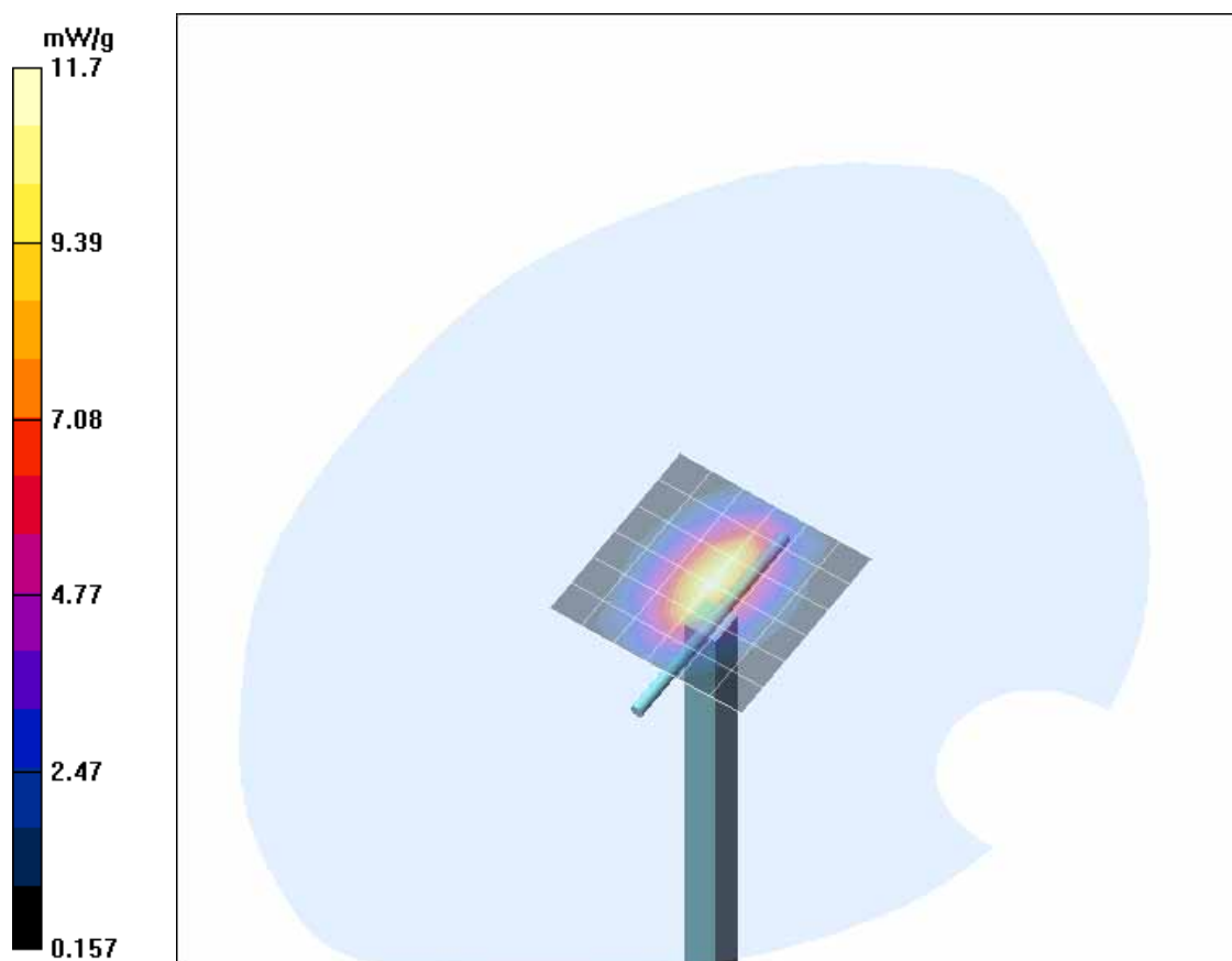
Fig. 15: Validation measurement 1900 MHz Body (July 21, 2006), coarse grid. Ambient Temperature: 22.0° C, Liquid Temperature: 21.3° C.
