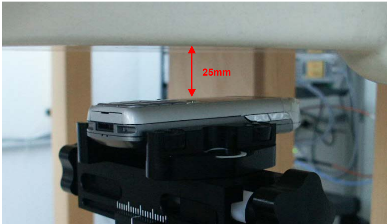
Fig. 27: Body worn configuration, PTT mode (Class 10), display towards the phantom.
