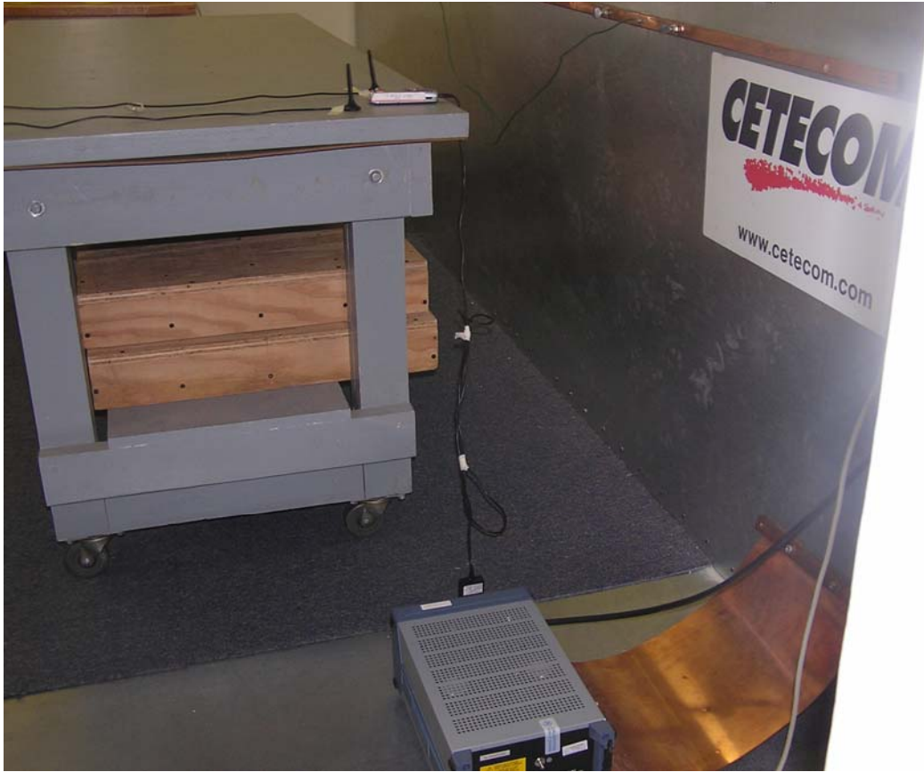
Test setup – AC Line conducted measurements
