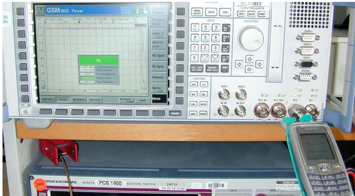
Fig. 2: Set up for conducted power measurement.
