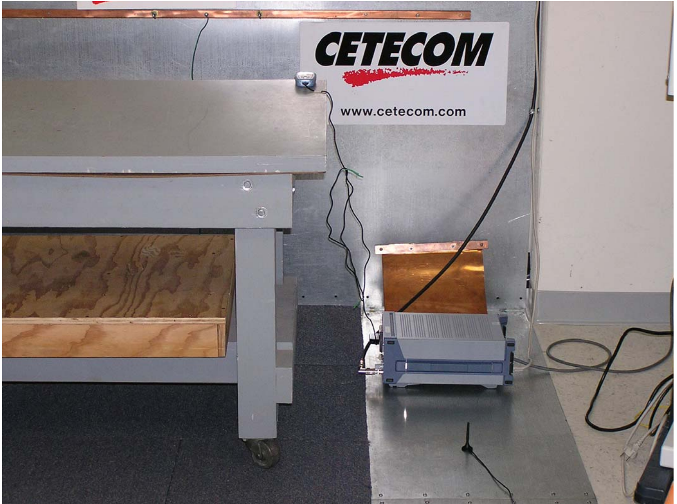
Test setup – AC Line Conducted Emissions
