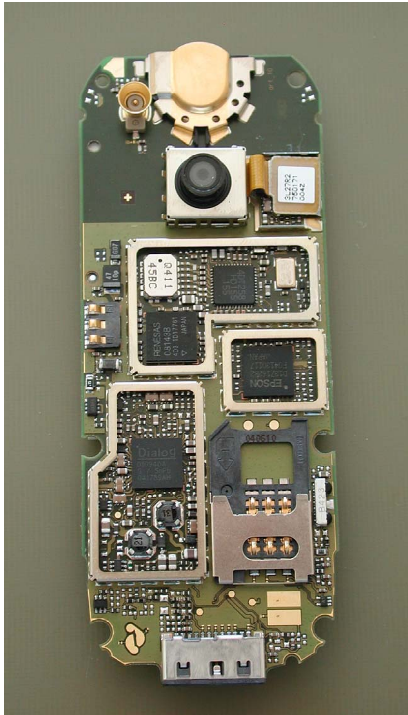
CX70E PCB Back View Shields Removed
