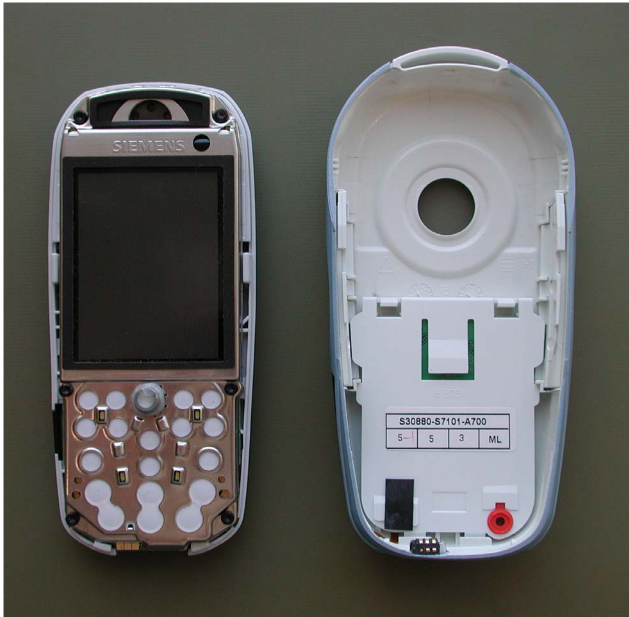
CX70E Disassembly Step 2
