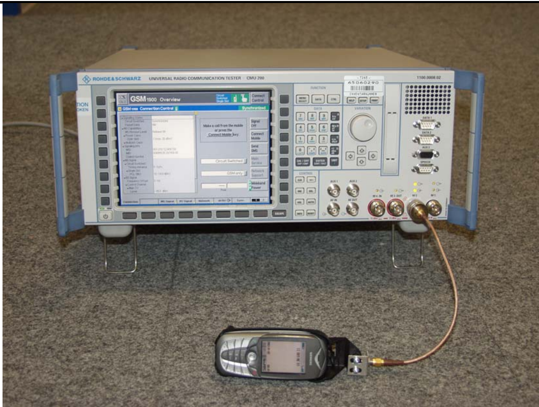
Figure 2: Set-up for conducted power measurement
