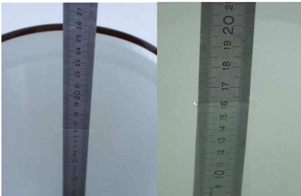
Fig. 55: Liquid depth for PCS 1900 Head and Body measurements.
