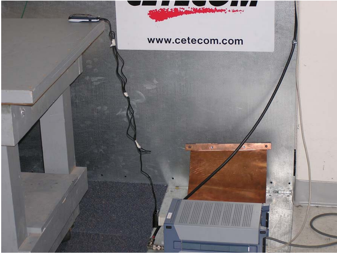
Test setup – AC Line Conducted Emissions
