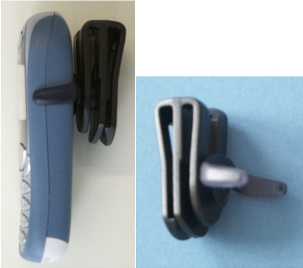
Fig. 18: Phone with used Belt Clip which dictates the closest distance to the body.
