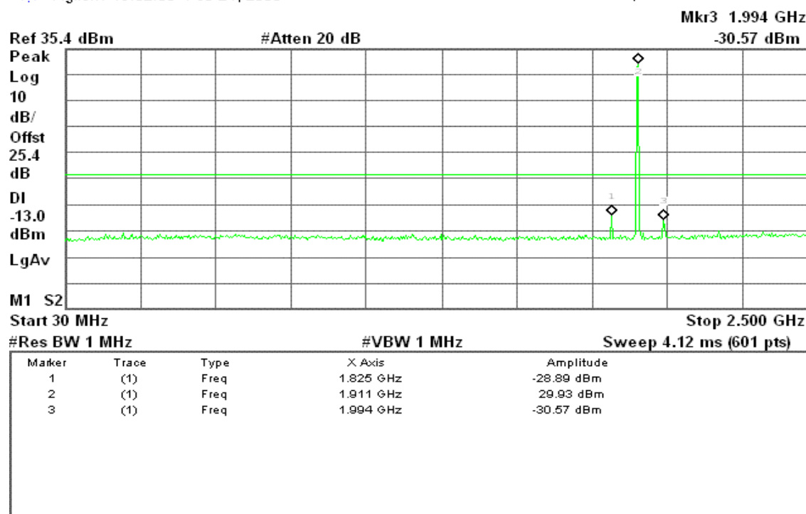
Figure 7-6: Out of Band emission at antenna terminals – GSM CH High
