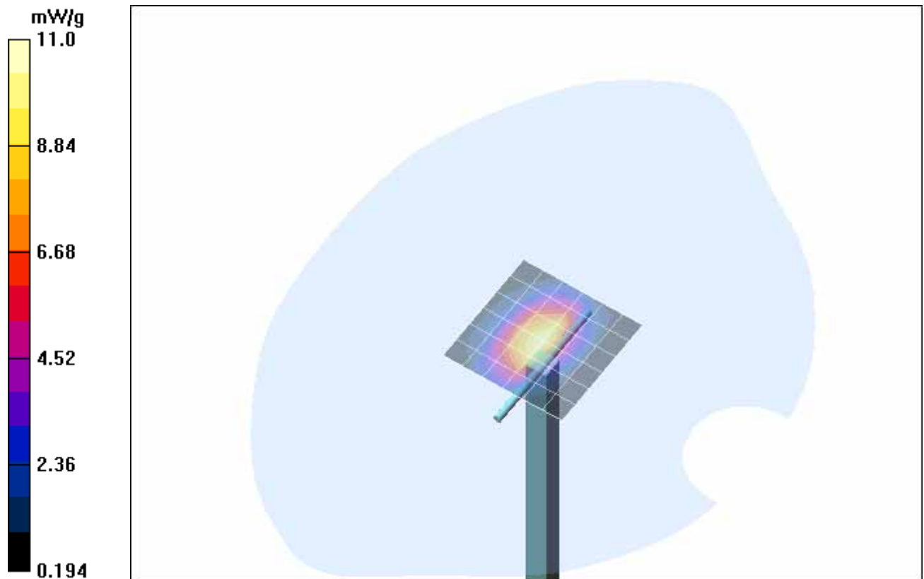
Fig. 14: Validation measurement 1900 MHz Head (August 22, 2005), coarse grid. Ambient Temperature: 22.0° C, Liquid Temperature: 21.0° C.
