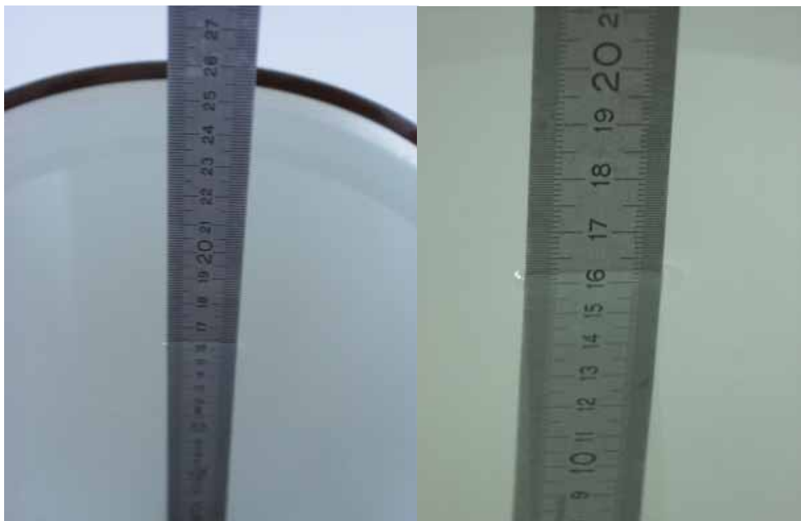
Fig. 38: Liquid depth for PCS 1900 head and body measurements.
