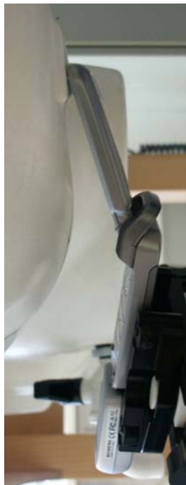
Fig. 24: Tilted position, left side, QuickPic Camera.
