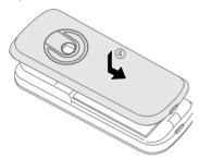
To remove, press the battery cover ⑤, and slide it off the phone ⑥.
