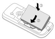
To remove, press the retaining tab on the side of the battery, then lift the battery out.  Place the battery cover on the phone slightly off centre 4 and then slide it until it clicks into place.
