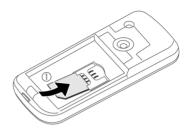
Insert the battery sideways into the phone ②, then press it downwards ③ until it engages.
