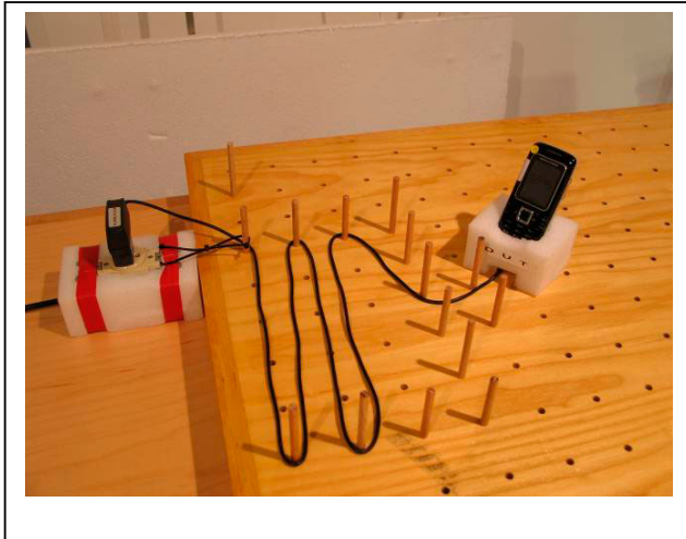
Figure 2.2 Conducted emission measurement with the travel charger in the range 0.15MHz to 30 MHz.
