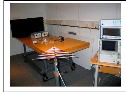
Figure 2.2 Conducted emission measurement with the travel charger in the range 0.15MHz to 30 MHz.
