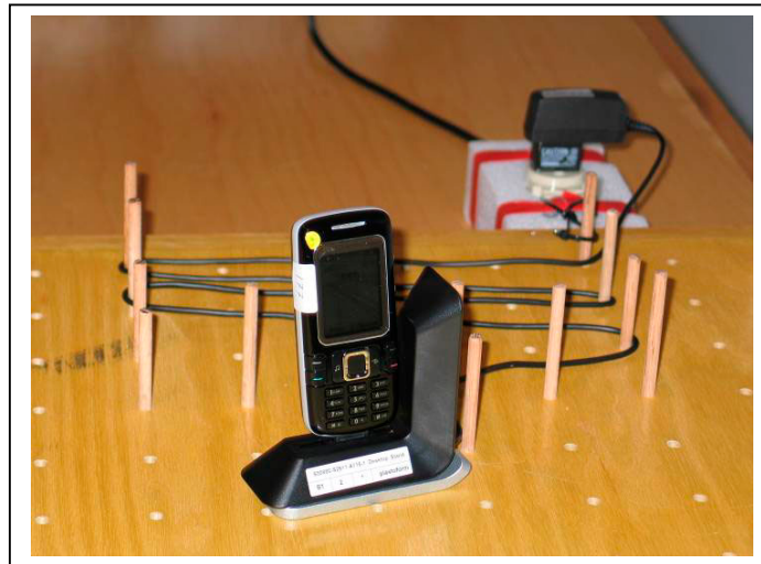
Figure 2.3 Conducted emission measurement with the travel charger US and desktop stand in the range 0.15MHz to 30 MHz.
