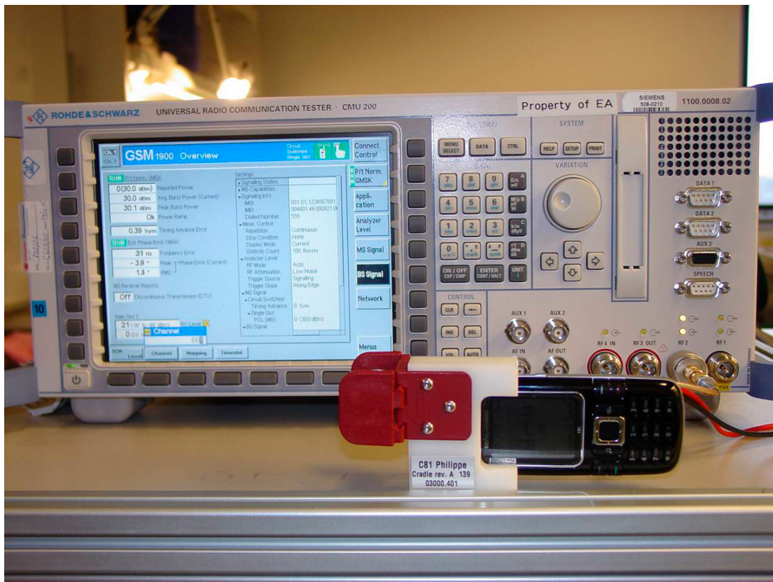
Figure 2: Set-up for conducted power measurement
