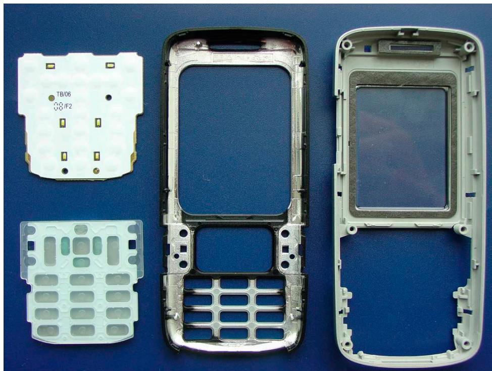
Disassemble Step 3: Front Cover disassembled
