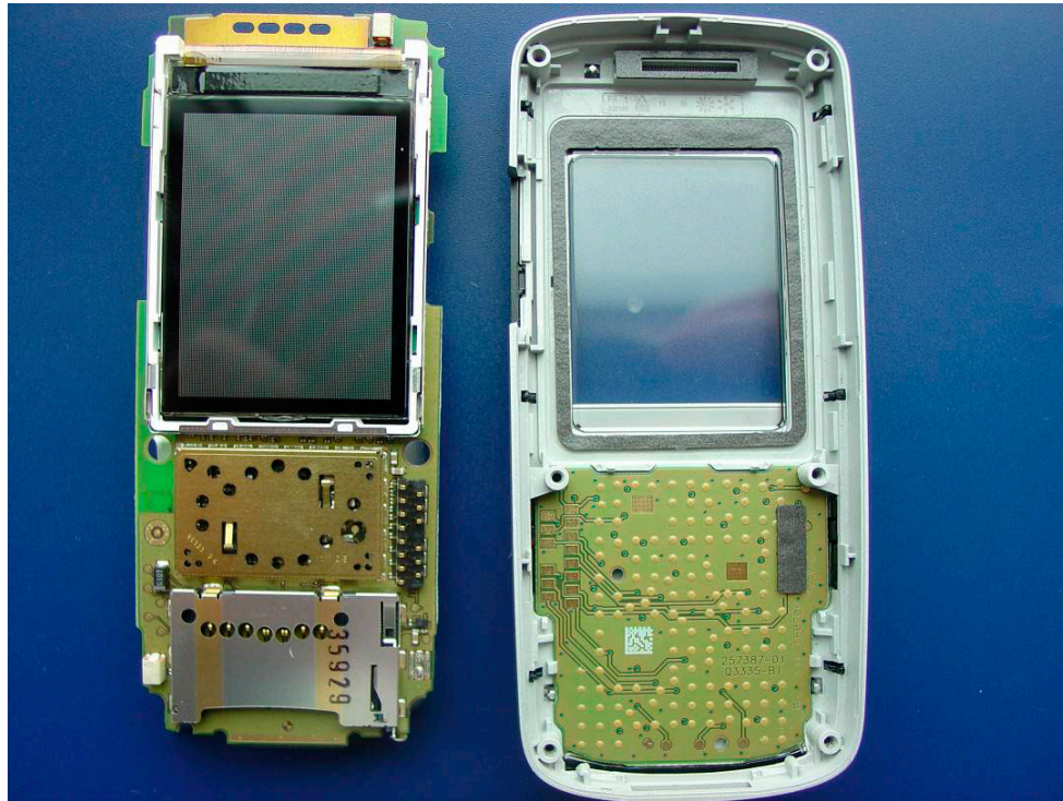
Disassemble Step 2: PCB separated from front cover
