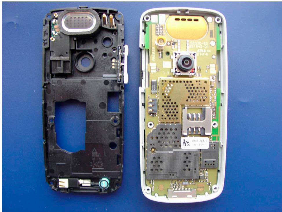
Disassemble Step 1: Lower Case opened
