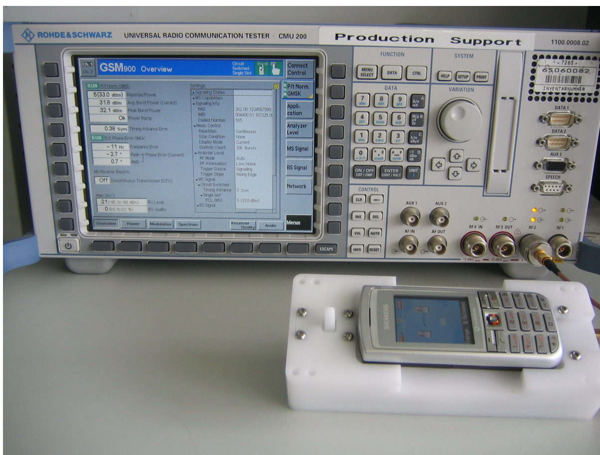
Figure 2: Set-up for conducted power measurement
