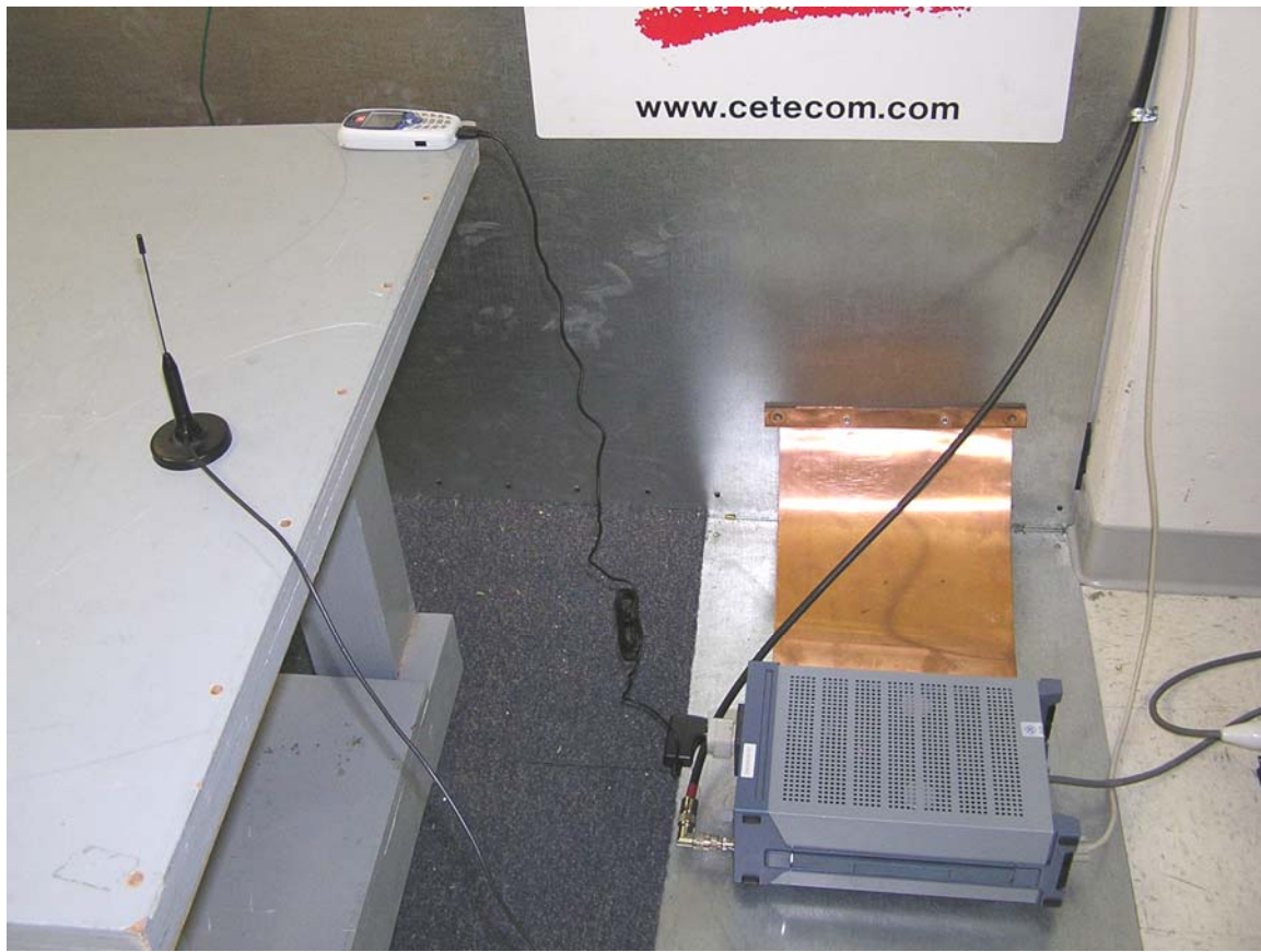
Test setup – AC Line Conducted Emissions
