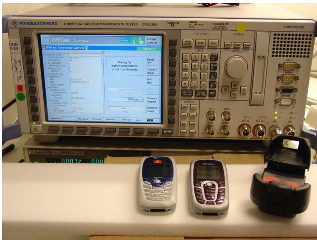
Figure 2: Set-up for conducted power measurement
