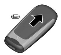
Insert the SIM card in the opening with the contact area facing downwards and push gently until it engages below the holder (make sure the angled corner is in the correct position 9mm).
