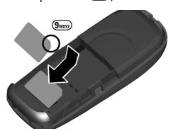
• Insert the battery sideways into the phone (9ww), then press downwards (9ww) until it engages.
