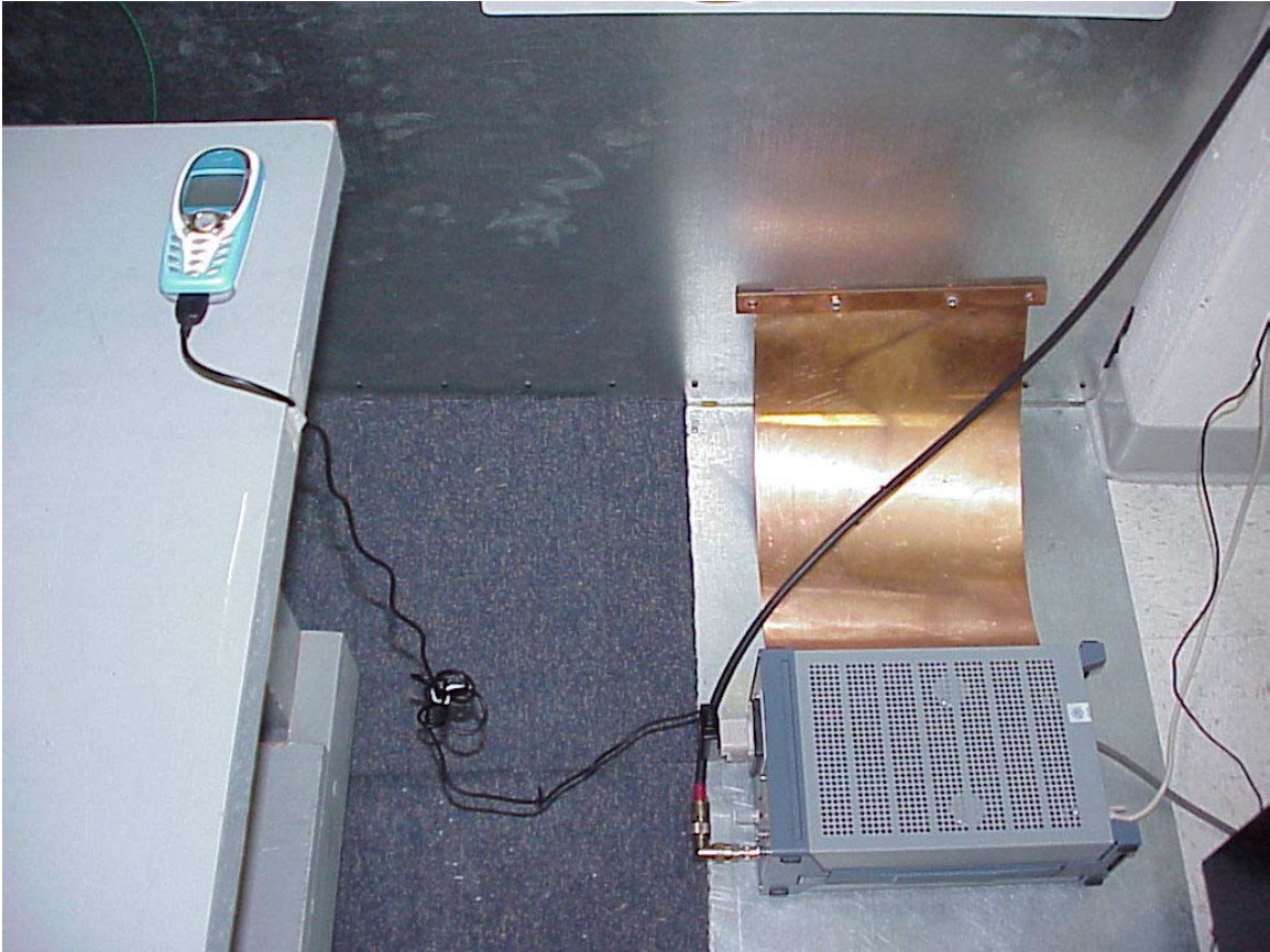
Test setup – AC Line Conducted Emissions
