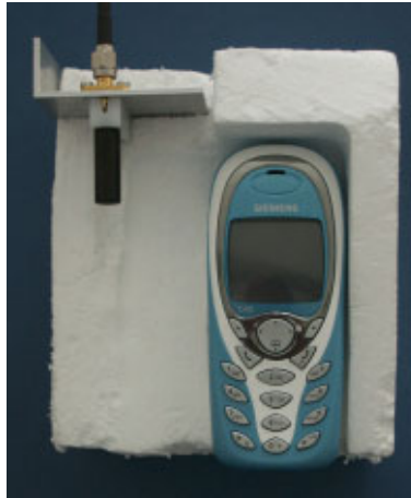
Fig. 8: Provided coupler to control the output power.
