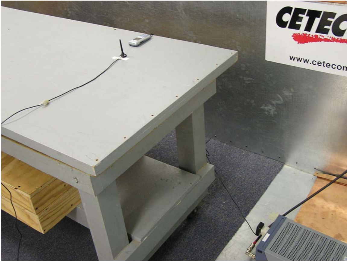
Test setup – AC Line conducted measurements
