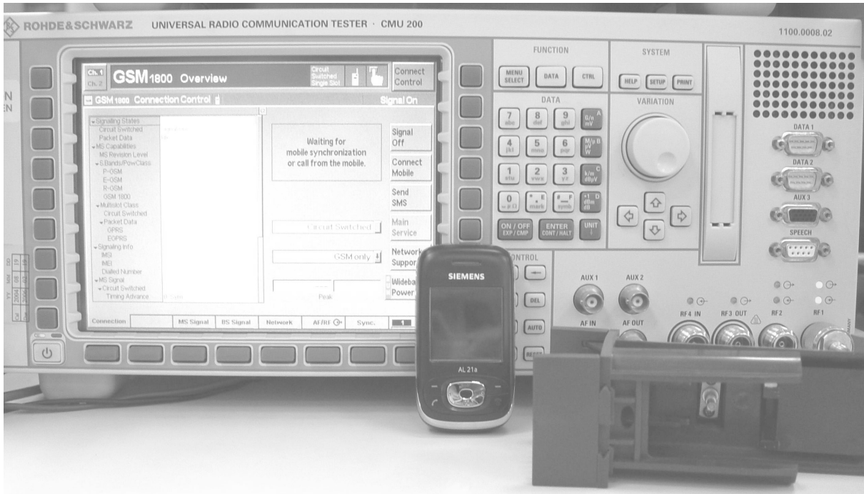
Figure 2: Set-up for conducted power measurement
