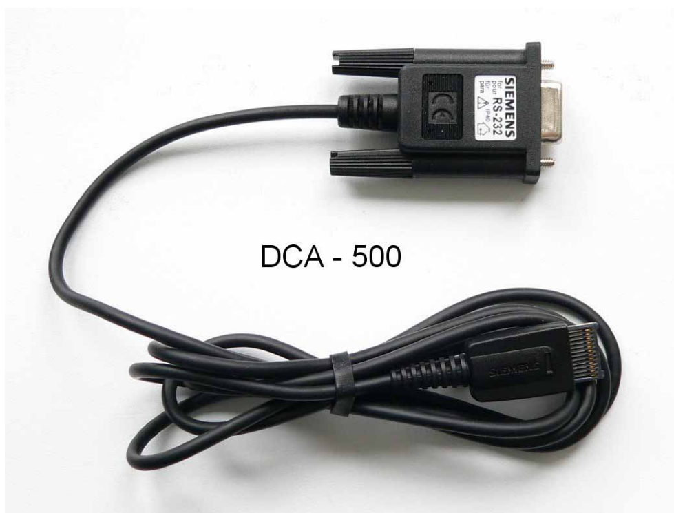
Fig. 17: Used data cable DCA-500.
