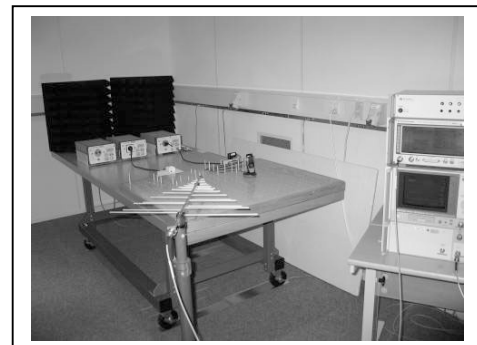
Figure 8.2 Conducted emission measurement with the travel charger in the range 0.15MHz to 30 MHz.
