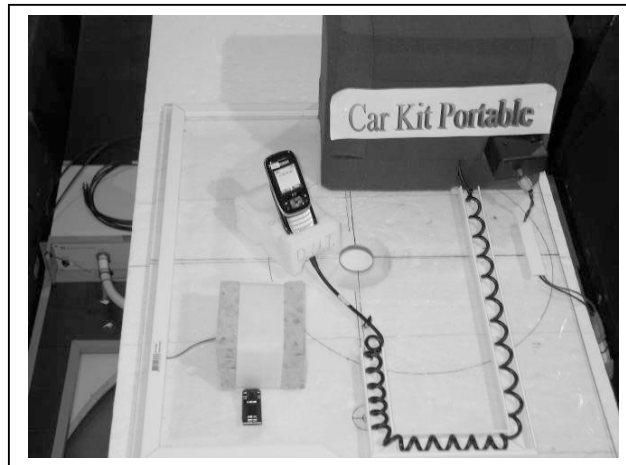
Figure 8.7 The setup for testing the Car Kit portable. The foam box contains the loudspeaker device due to the fact that the setup is also used for immunity test with respect to the European standards.
