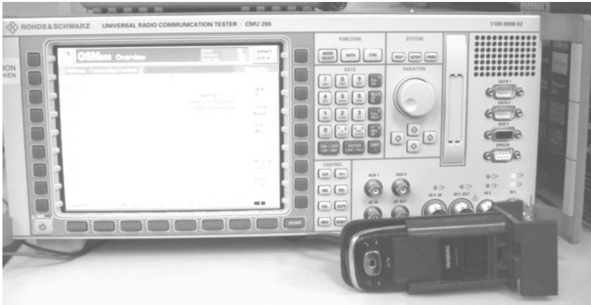
Figure 2: Set-up for conducted power measurement
