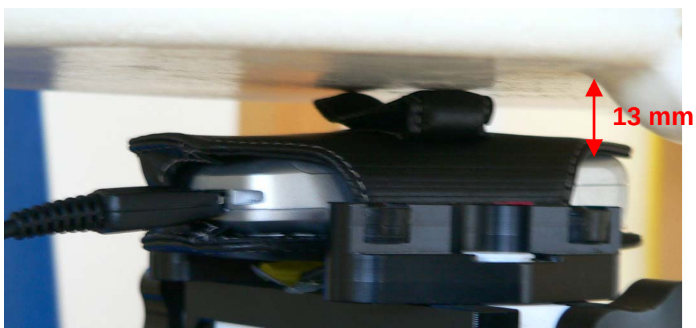
Fig. 30: Body worn configuration, GPRS mode (Class 8) with data cable, antenna towards the phantom and FCL 600 carry case.
