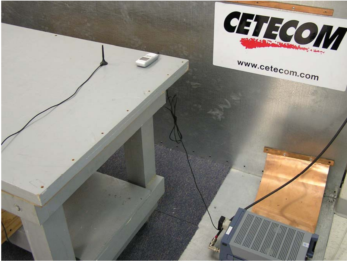
Test setup – AC Line conducted measurements
