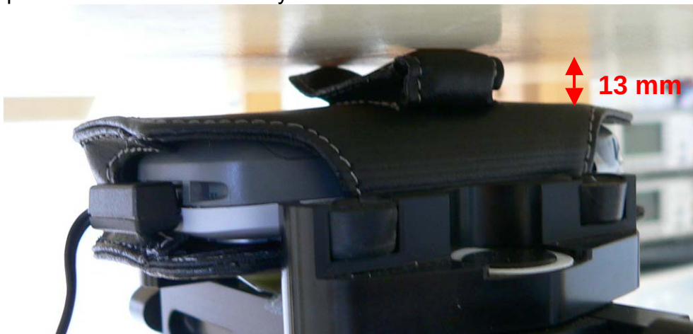
Fig. 30: Body worn configuration, GSM mode with headset, antenna towards the phantom and FCL 600 carry case.
