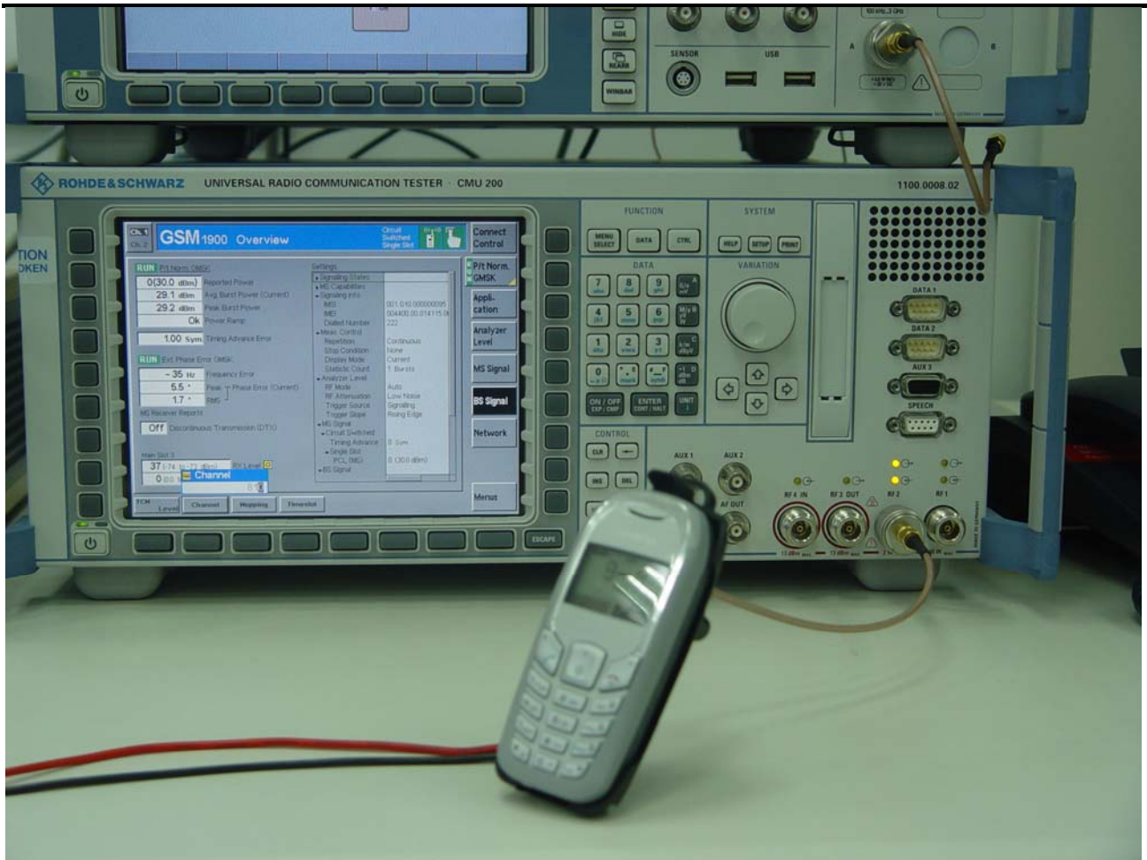
Figure 2: Set-up for conducted power measurement
