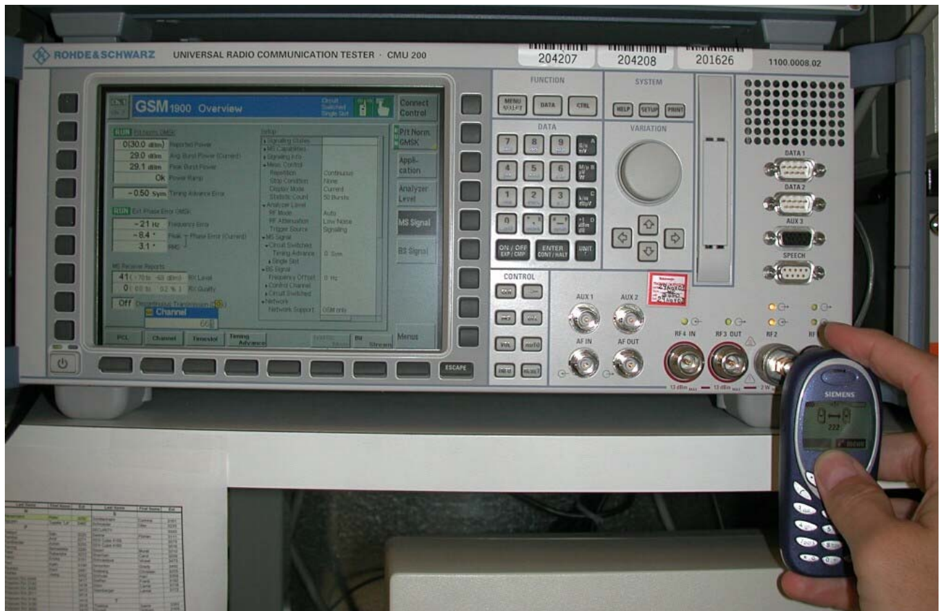
Fig. 2: Set up for conducted power measurement
