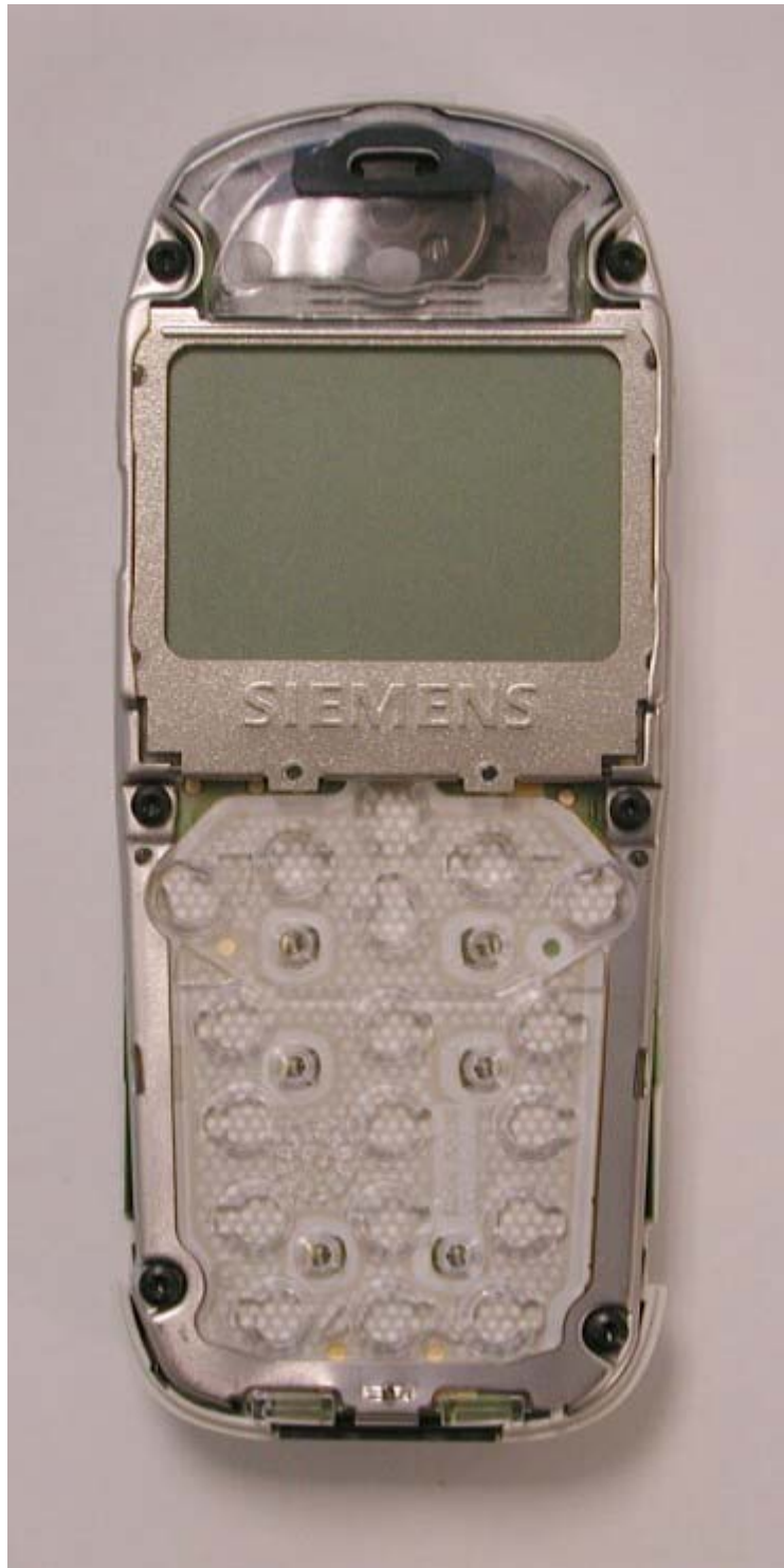
A56 Front cover removed
