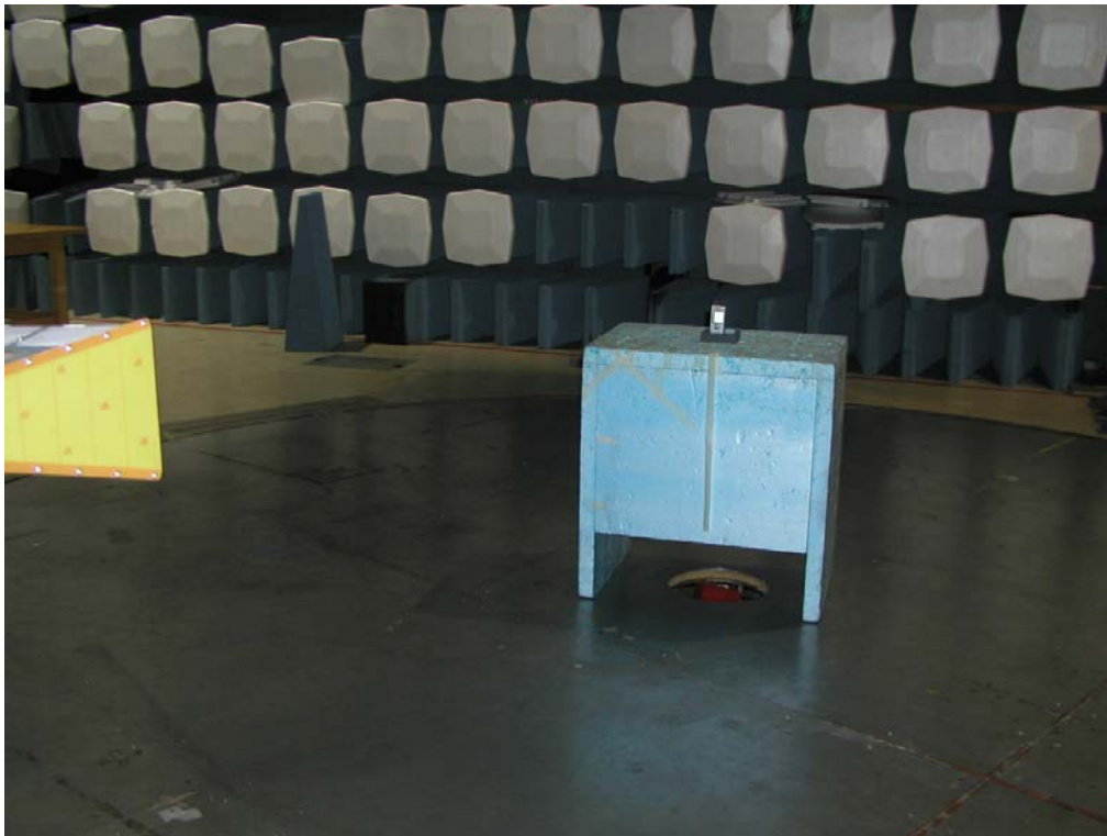
Photograph 1. Radiated RF output power test setup
