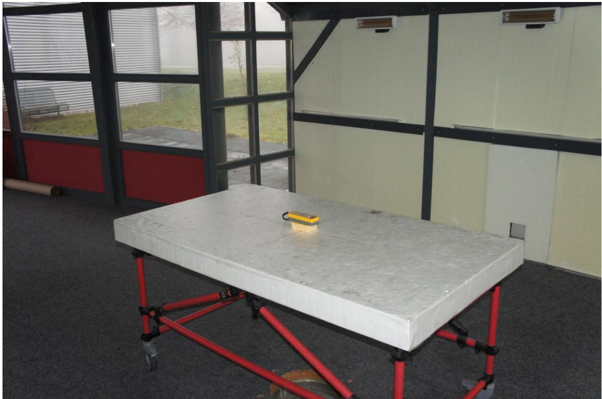
Picture 7: EUT test setup in open area test site (rear view)
