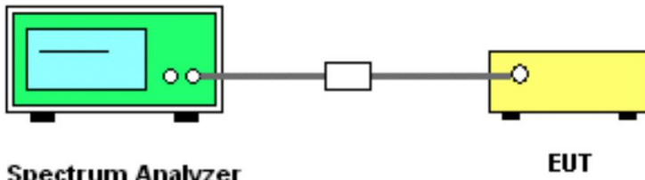
Picture 32: Test setup for conducted spurious emission measurement
