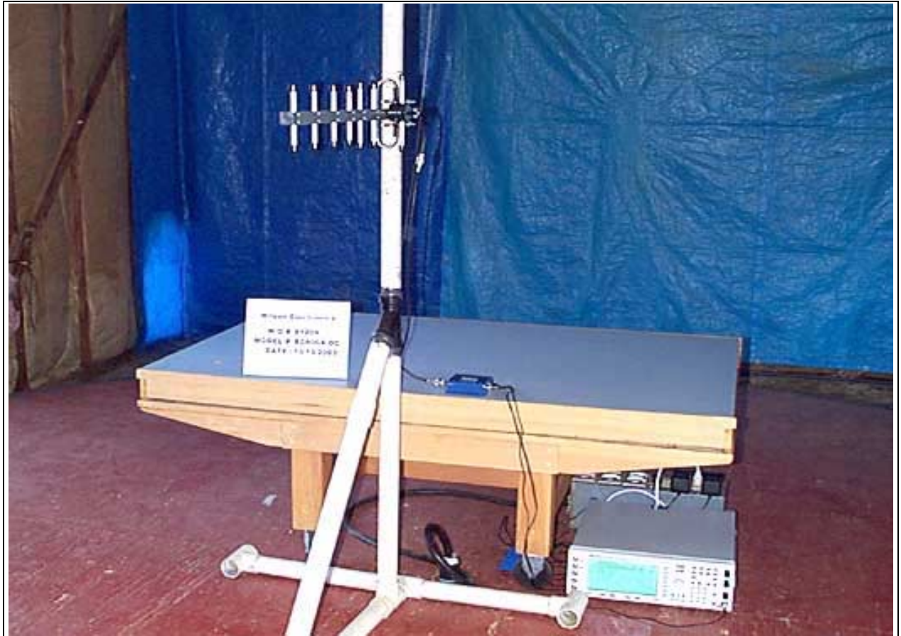
Radiated Emissions with 13 dBi Yagi Antenna
