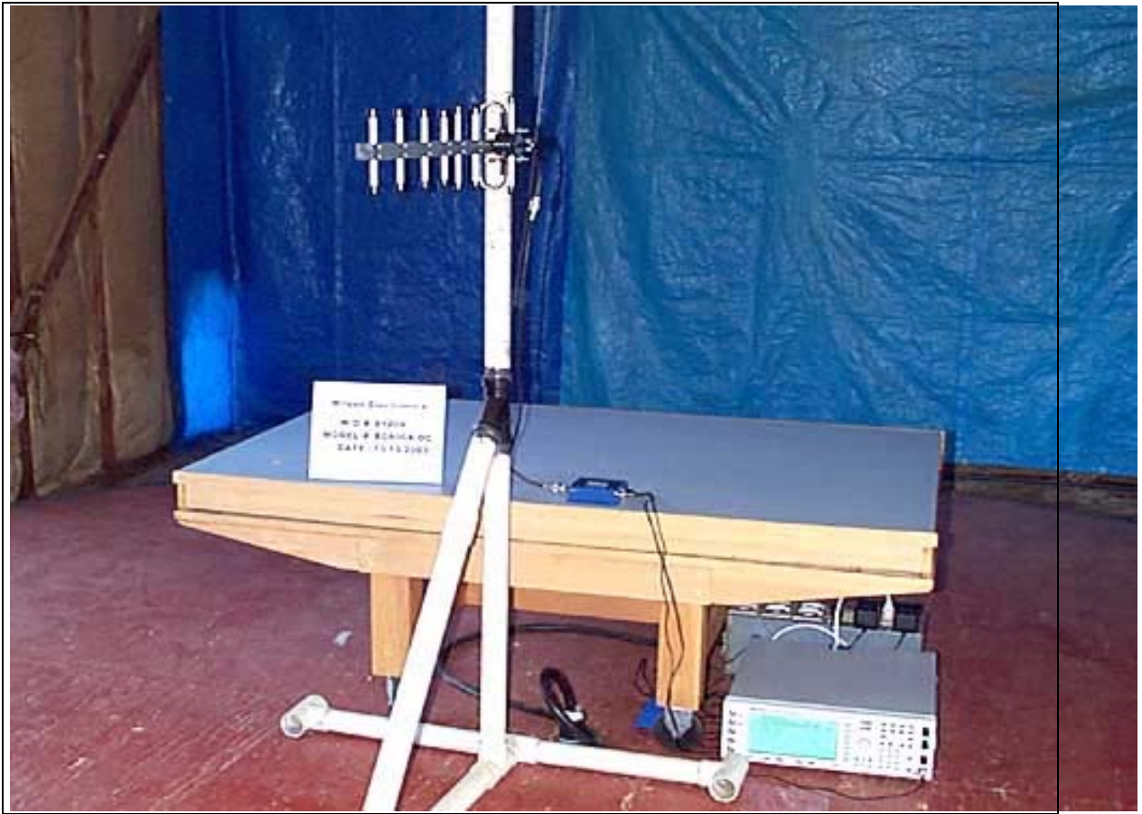
Radiated Emissions with 13 dBi Yagi Antenna
