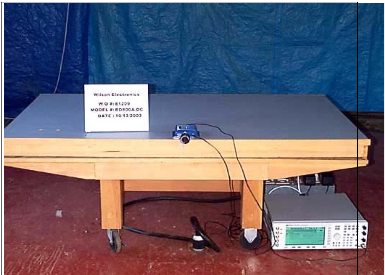
Radiated Emissions with Downlink RF Port Terminated
