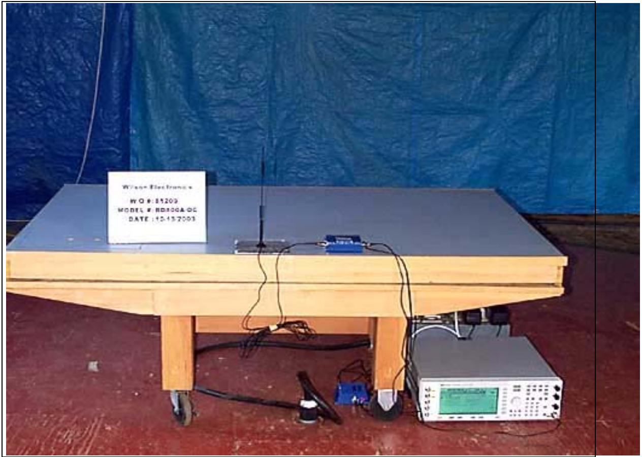
Radiated Emissions with 5 dBi Whip Antenna
